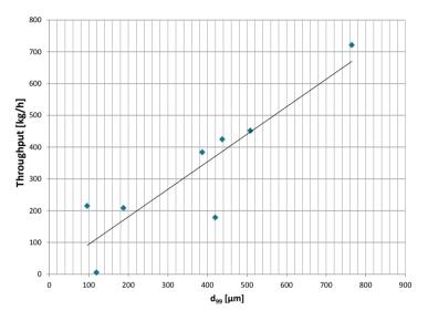
Lactose grinding with the Impact Mill Condux® 300
