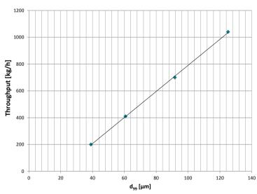
Lactose grinding with the Classifier Mill CSM 360
