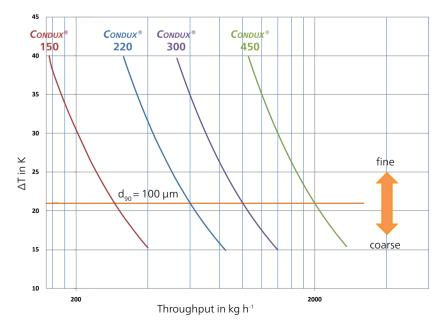
Sugar-grinding with impact mill CONDUX® COMPACT
